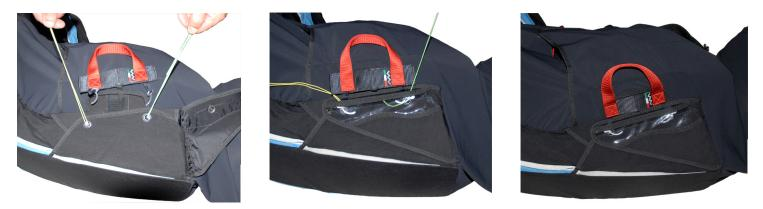
Push the metal pins on the handle into the elastic loops and under the transparent cover. It is essential to remove the cords after this operation. The cords should be pulled out slowly in order not to damage the elastic loops by excessive friction. Lastly, the handle should be positioned under the elastic cover.
